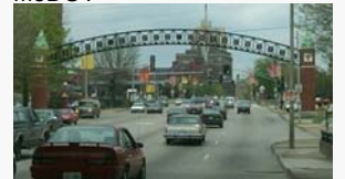
P-B.2: Design elements spanning across the street will not be permitted by MoDOT
