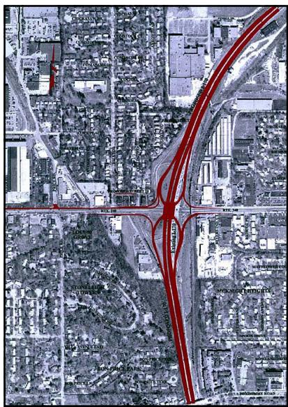
The Olive/I-170 interchange is currently being reconstructed by the Missouri Department of Transportation (MODOT). The project consists of relocating the interchange, widening the ramps to and from the interstate, and widening Olive Boulevard under I-170. This project, which will reduce congestion in the area, is expected to be complete in late 2007.
